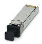
The small form-factor plug-in module provides a fiber optic interface with a data transmission speed of 100 Mbps with a wavelength of 1310 nm (long).
